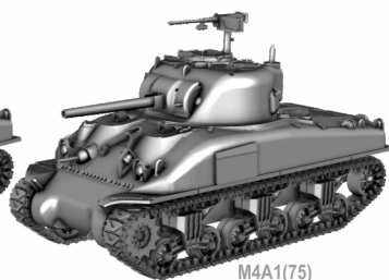
M4A1(75) Small hatch, 75mm gun with M34A1 mantlet, high bustle turret, and T48 track links.
