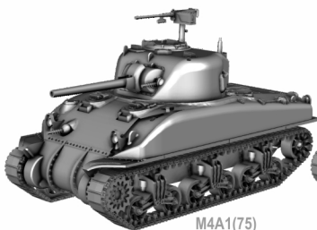
M4A1(75) Direct vision port, 75mm gun with M34 mantlet, low bustle turret, and T41 track links.
